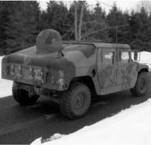
Figure 15. Ka-band (satellite-based broadband) mobile SATCOM on the move
