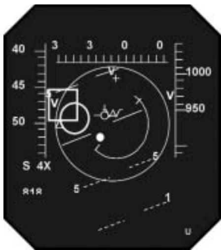
Figure 1. An F-15C's HUD. (Reprinted from Maj Reid Cooley, briefing, subject: Joint Helmet-Mounted Cueing System, 422d Test and Evaluation Squadron, Nellis AFB, Nevada, June 2001.)
